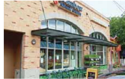
A good example of a storefront that animates the street edge and sustains a pedestrian's interest with a high degree of transparency along the street, through which uses are readily discernable to the passer-by. Overhead cover along the sidewalk and seating adds pedestrian comfort.
