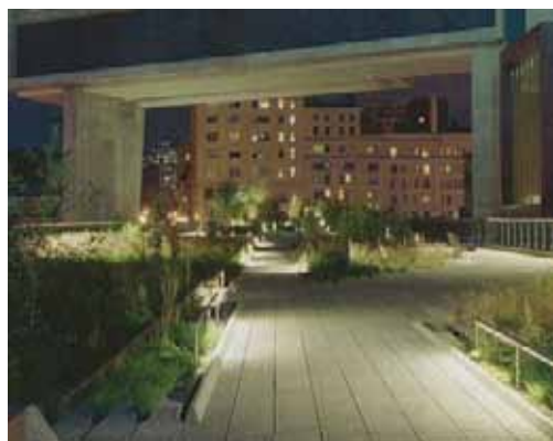
Handrail integrated light fixtures
