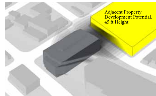
In Transect L5, shading of the development potential on adjacent properties is limited to 15 meters (~49 feet). The yellow block north of the project site represents the 45 ft zoning envelope. Shadows cast by 3400 Stone Way fall well below the roofline.
