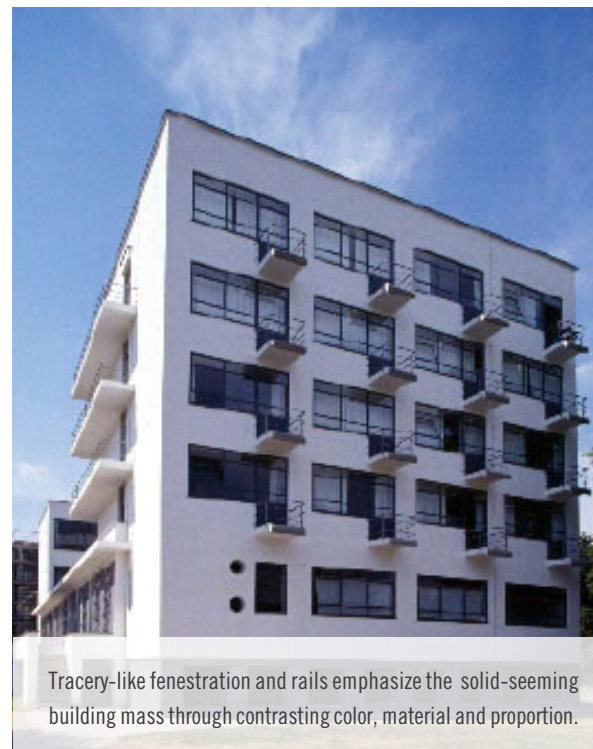
The window wall has a basic A-B bay structure that appears whimsical and complex due to localized variations in the mullion patterns.
