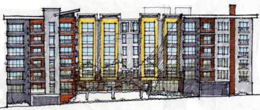
FACADE STUDY SHOWING ERODED BUILDING MASSES WITH TOWER ELEMENTS, VERTICAL CHIMNEY ELEMENTS, PROJECTING BAYS, UNIQUE CHARACTER AT BUILDING WINGS, AND UNIQUE CHARACTER AT THE COURTYARD FACADE
