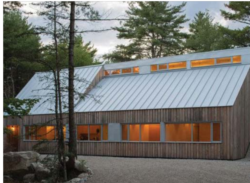
AEP SPAN "STANDING SEAM METAL" - EXAMPLE
