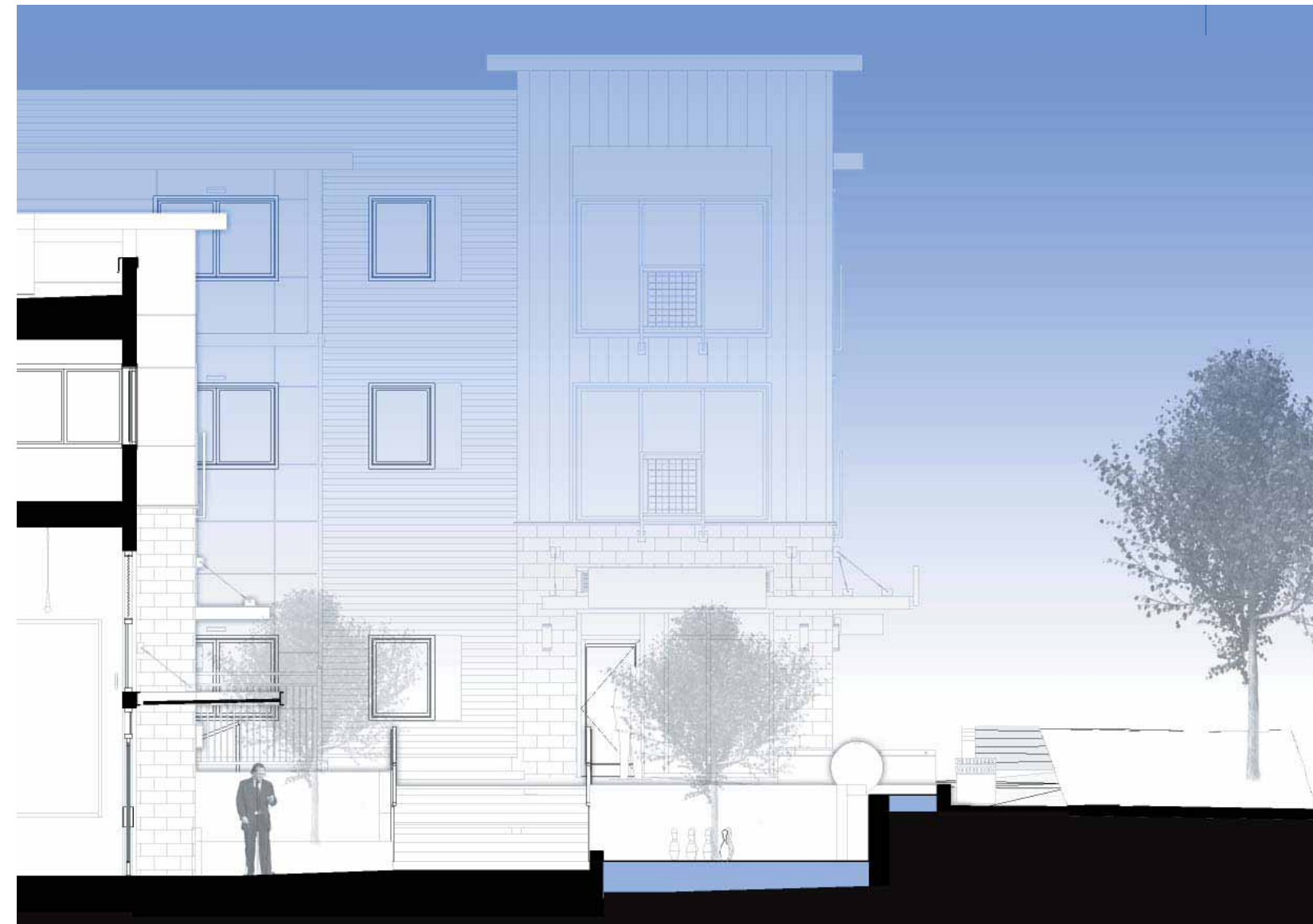
LEASING OFFICE 23'-0" ENTRY PLAZA 24'-0" WATER FEATURE / AMENITEY PLAZA 6'-6" SIDEWALK 6'-0" PLANTING STRIP SECTION A - TYPICAL SOUTH BUILDING PLAZA ALONG GREEN-
