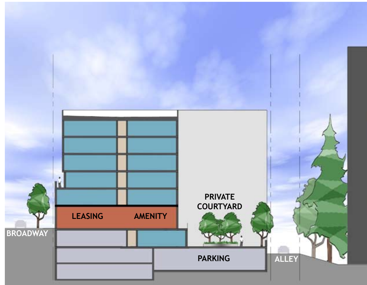
CROSS SECTION THROUGH COURTYARD
