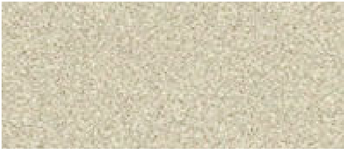
CEMENT PLASTER COVERED EPS FOAM WITH INTEGRAL COLOR COLOR: MATCH PATTERSON WHITTAKER "TUSCAN" LOCATION: ALL TRIM, CORNICES AND WINDOW SURROUNDS ON MASONRY & STUCCO
