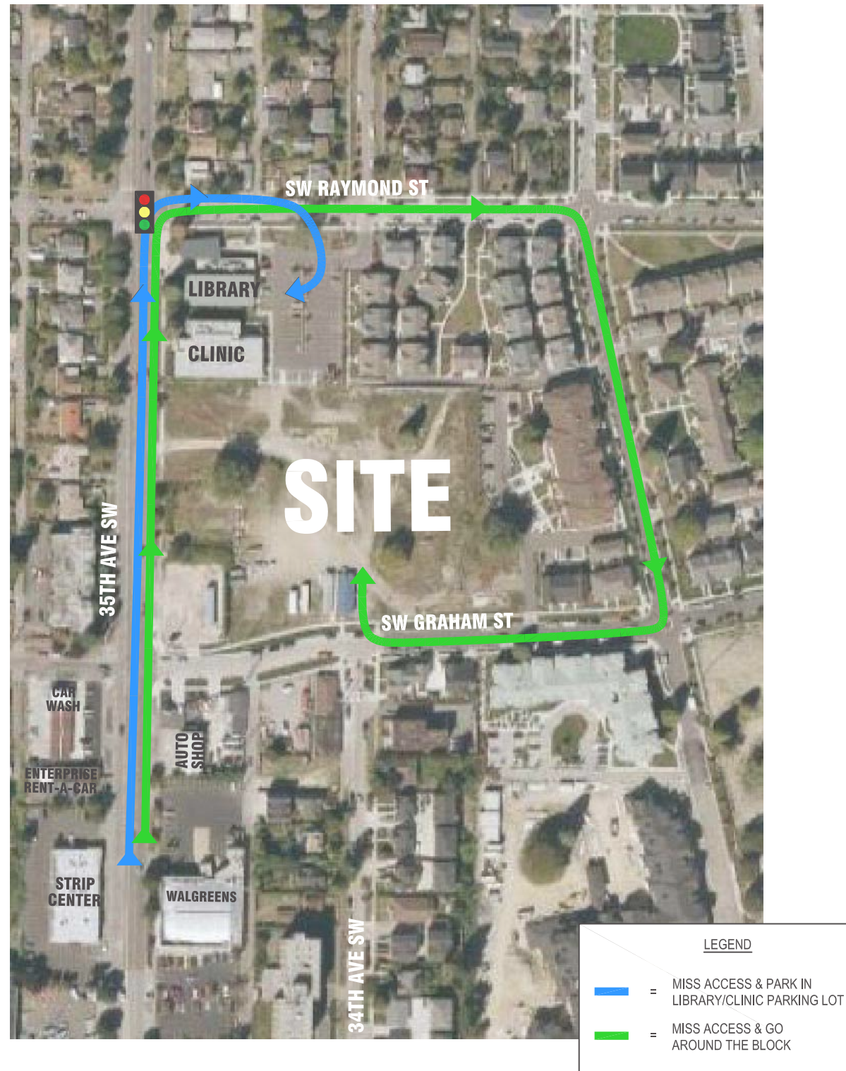
Circulation patterns modeled by Transportation Engineer model 1 no retail entrance off 35th Ave. SW
