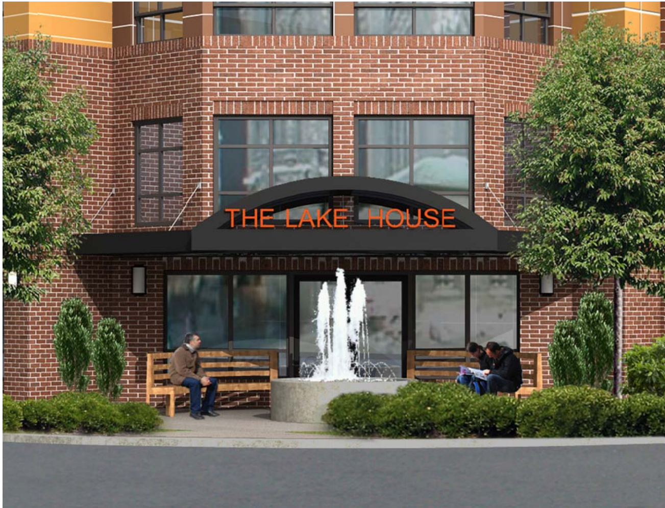
Main Residential Entry Canopy Dark anodized aluminum with a combination of glass and solid infill
