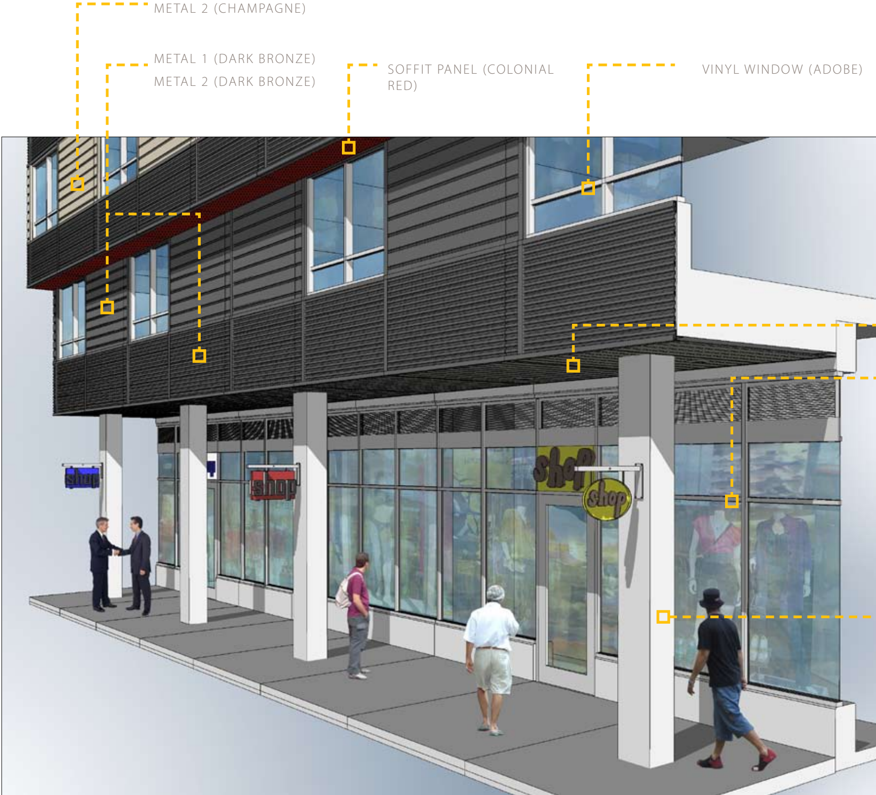
STOREFRONT & SOFFIT DETAIL AT 11TH AVE FACADE
