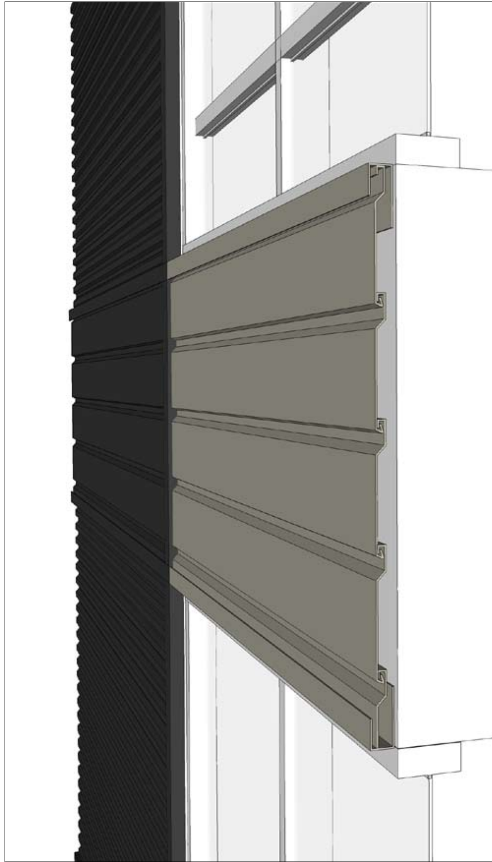
DETAIL OF METAL SIDING
