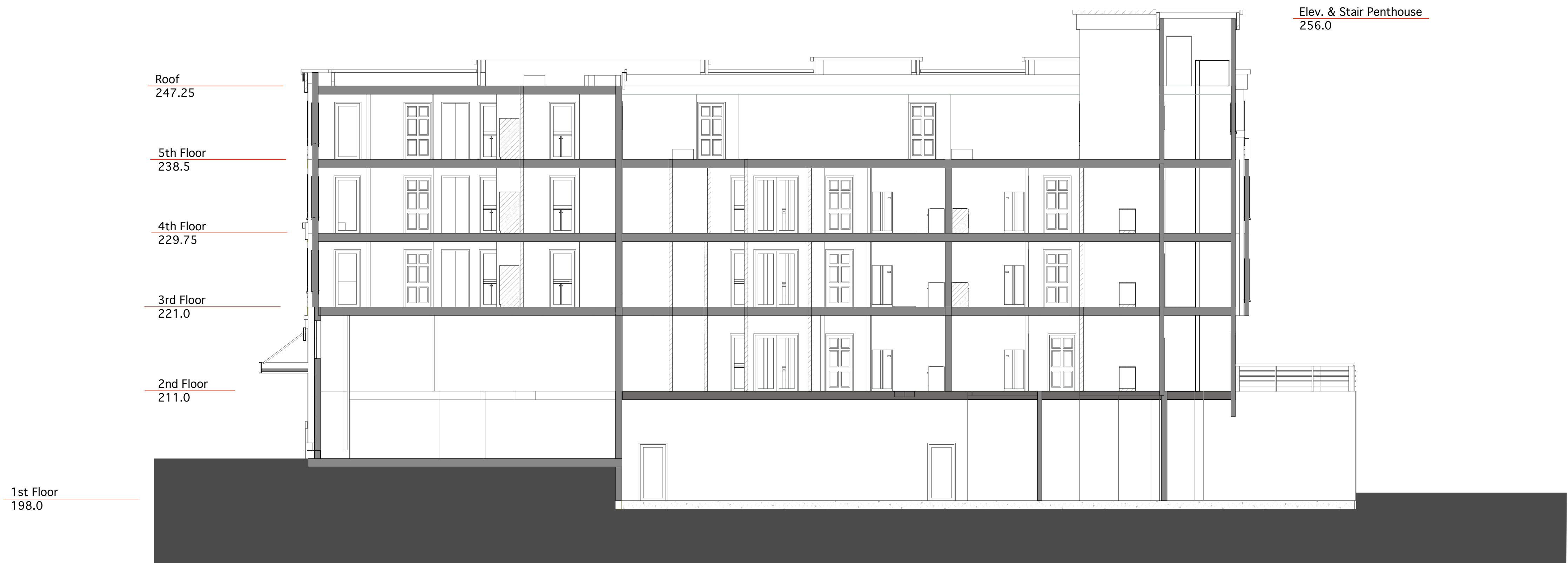
BUILDING SECTION A-2 EAST/ WEST 1/8" = 1'-0"
