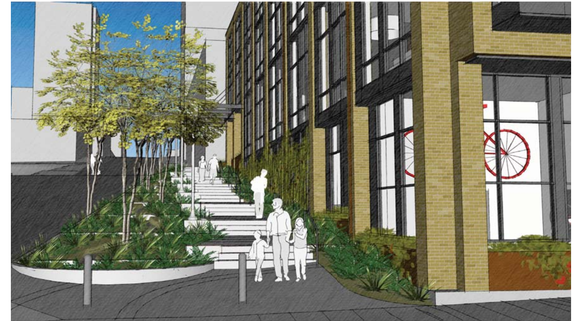
AFTER - showing current scheme. Note relocation of watercourse to street edge, straightening of steps, gravity-fed system (instead of a recirculating "fountain"), and vertical runnels inset in brick columns.
