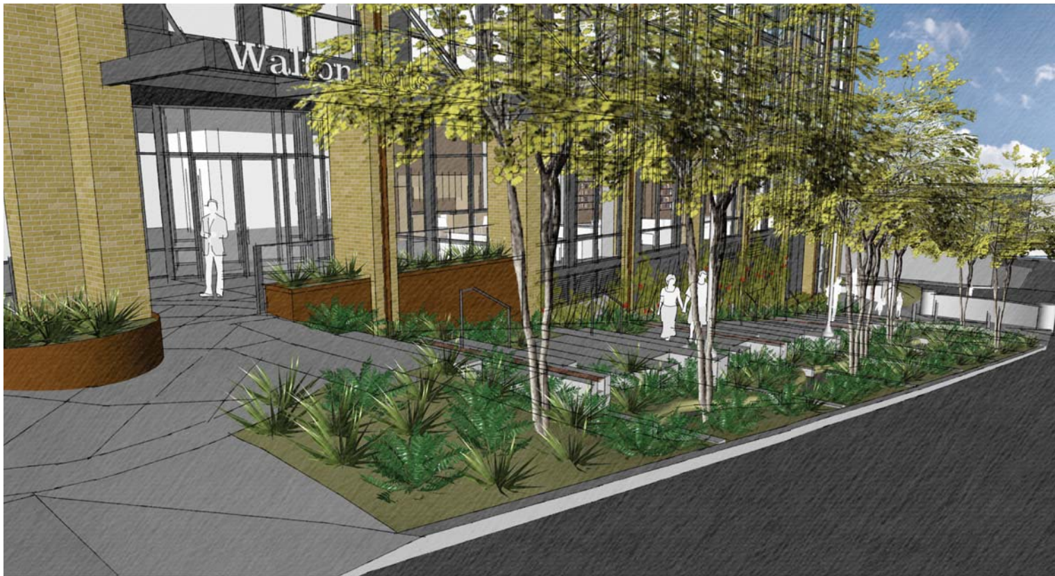
Head of rain garden watercourse. All detained roof water will be released to this point as well, resulting in a longer-duration flow of water through the rain gardens toward the Cistern Steps.
