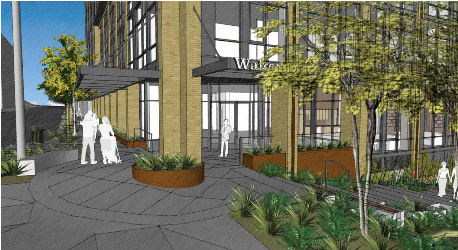
Corner of Western Avenue and Vine Street. Note Cor-ten steel planters, vertical runnel / downspout within brick column and conveyance across sidewalk to rain gardens and weirs.
