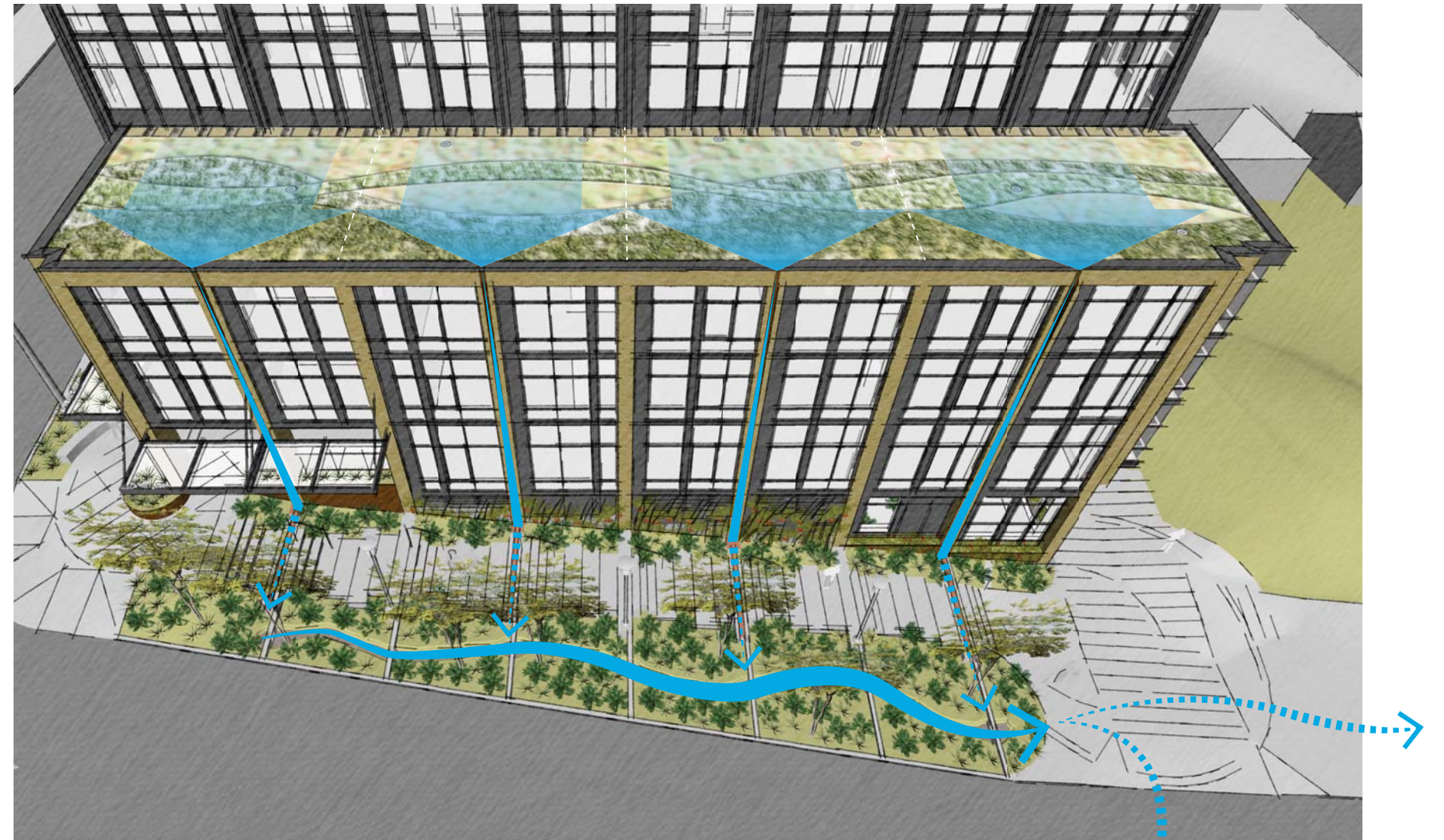
above: diagram illustrating drainage of view corridor green roof below: images of conveyance across sidewalk to rain gardens / weirs
