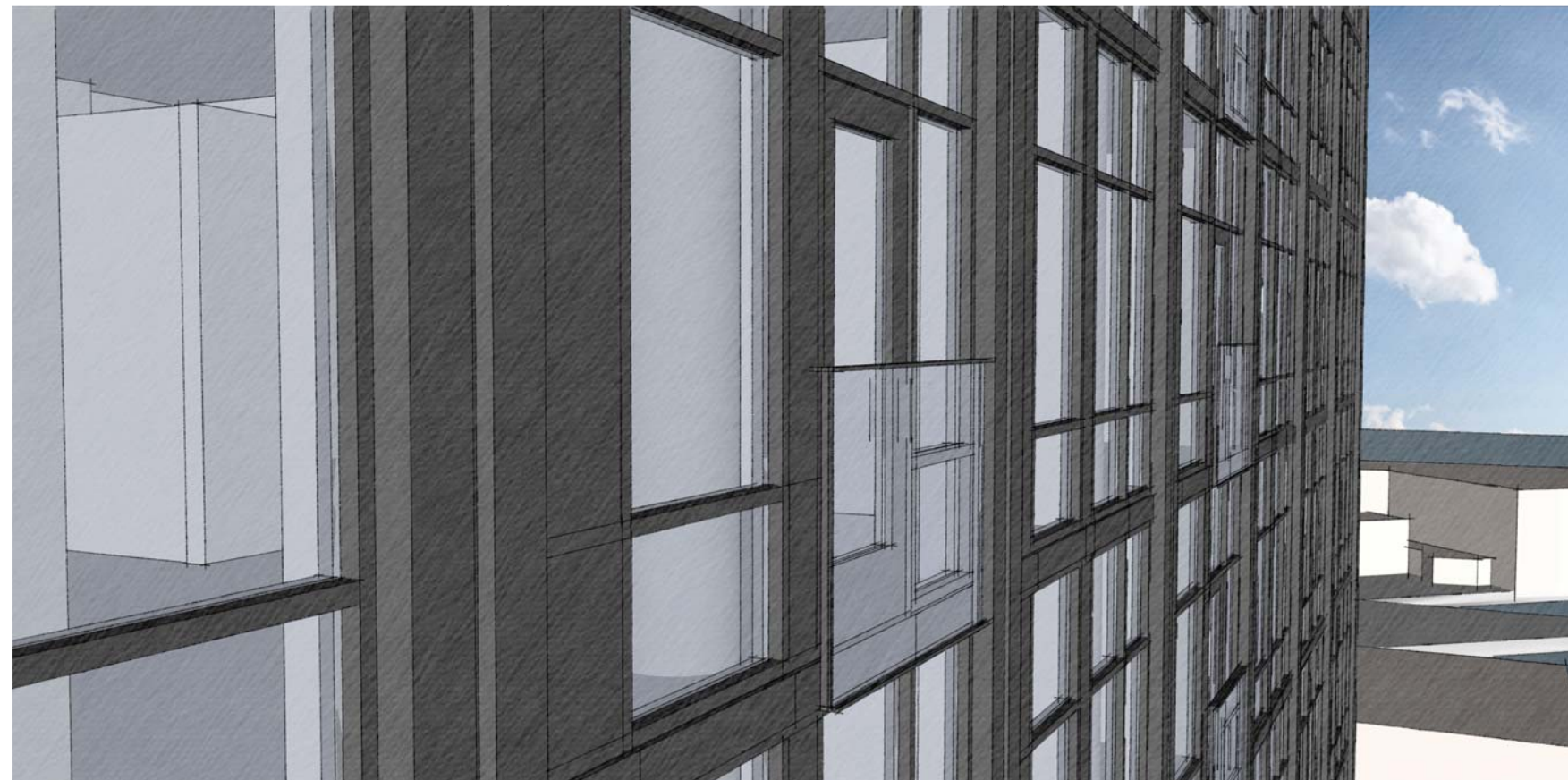
VIEW CORRIDOR DECK @ NORTH FACADE - detail showing "juliet" balconies at view corridor
