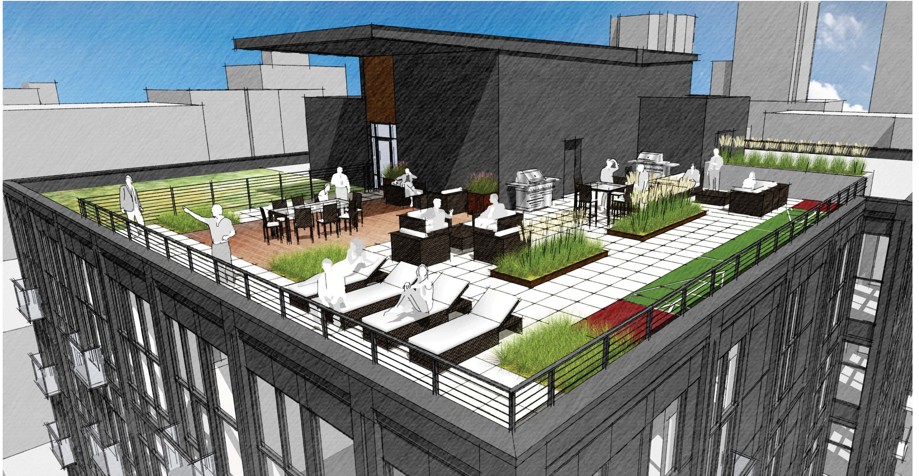
above: rooftop amenity space with gathering areas, barbeques, planting, green roof and shuffleboard court. Note rooftop mechanical equipment located toward center of roof, with larger elevator penthouse mass broken by smaller mechanical screens, electrical room, boiler room and shaft pressurization fans enclosure.
