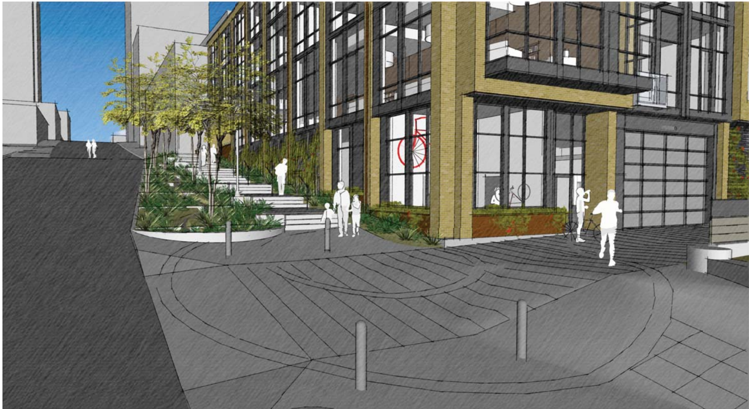
Base of rain garden watercourse. Water reaching this point may be conveyed to the Cistern Steps, with the permission of those responsible for that private system, otherwise it enters the City's storm drainage at this point.
