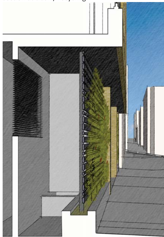
section at transformer vault / venting green screens
