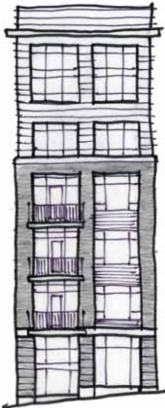
Metal siding spandrels between windows (PROPOSED)
