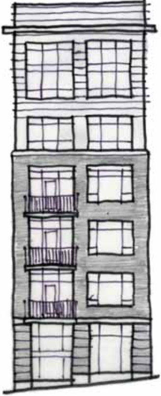
Brick spandrels between windows (ALTERNATE)
