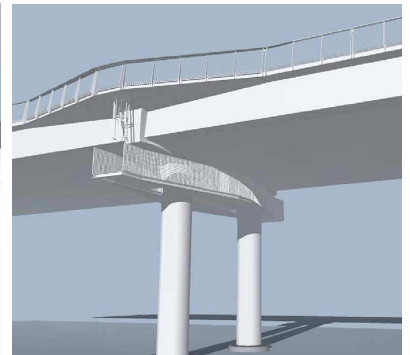
belvederes & maintenance catwalks
