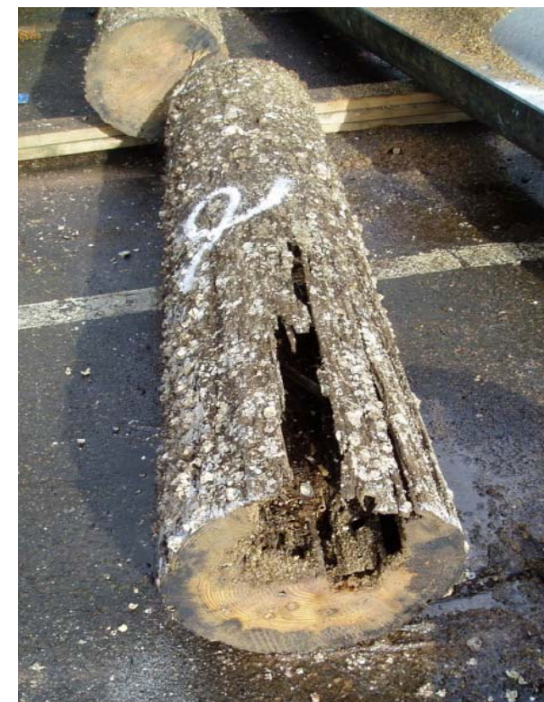
Timber pile from Colman Dock that has been removed and replaced due to deterioration.
