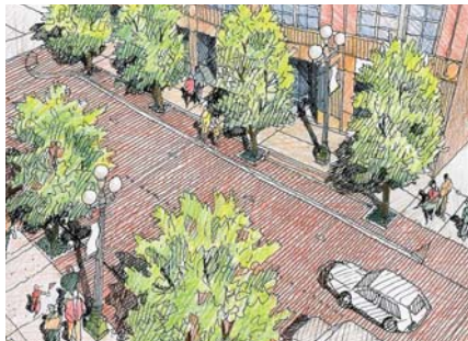
Street trees, wide sidewalks, and varied pavement color and texture make it clear where pedestrians and vehicles are to travel, thereby reducing the potential for conflicts between them.
