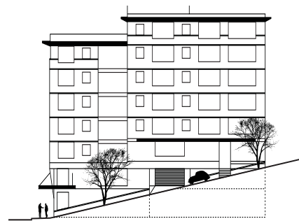
The topography of a relatively steep site is expressed through the form of the building and its stepped roofline.
