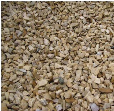
Crushed stone path/ Access (± 1/4" minus material)
