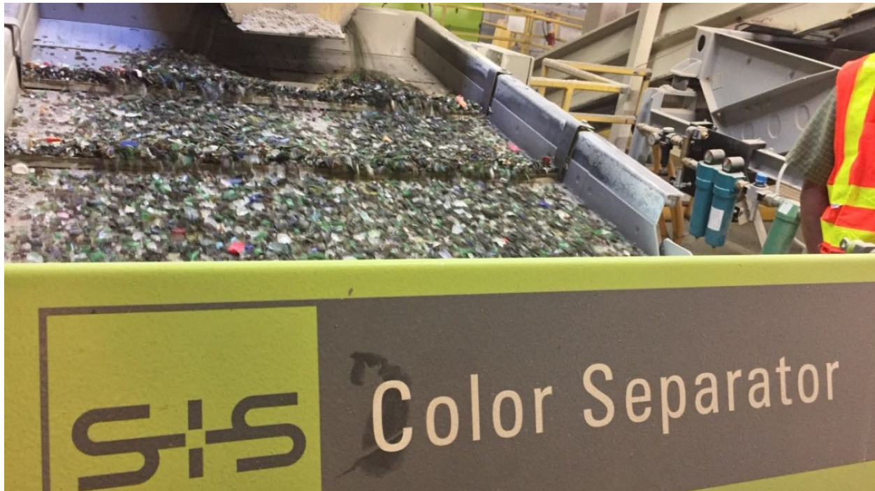
Glass sorted by color for recycling at Strategic Materials, Inc. in Seattle (Source: SPU Image Library)
