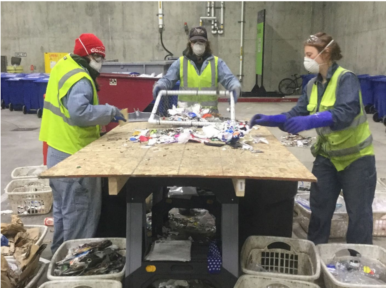
City contractors sort residential waste to measure capture and contamination rates (Source: Cascadia Consulting Group)
