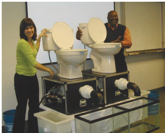
Molly Brumley of Colehour+Cohen and Arece Hampton of SPU compare the performance and water use of a 3.5 gallon toilet with a new 1.28 gallon WaterSense model.
