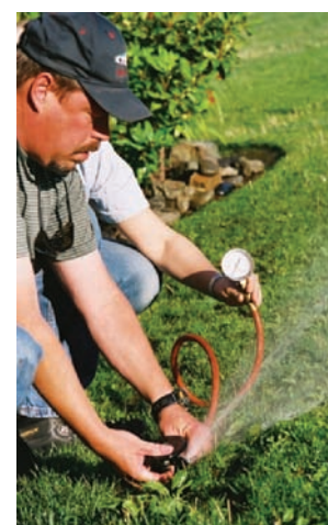
Contractor checking an irrigation system.
