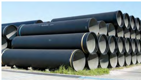
Example of Schematic of Earthquake Resistant Ductile Iron Pipe (ERDIP) used for earthquake emergency.
