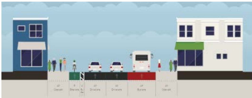
Figure 15 Downtown Proposed Cross-Section of Spring Street Between 2 nd Avenue and 3 rd Avenue (looking east)
