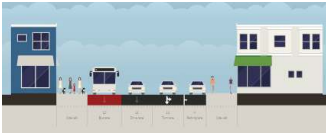
Figure 14 Downtown Proposed Cross-Section of Madison Street Between 2 nd Avenue and 3 rd Avenue (looking east)
