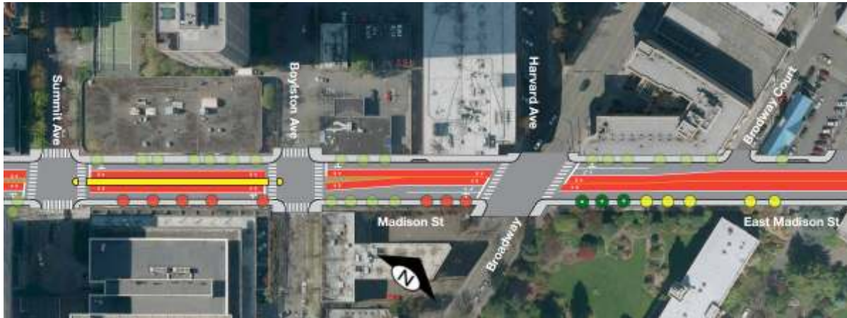
Figure 16 First Hill Segment - Madison Street with Left Turn and Transit Channelization
