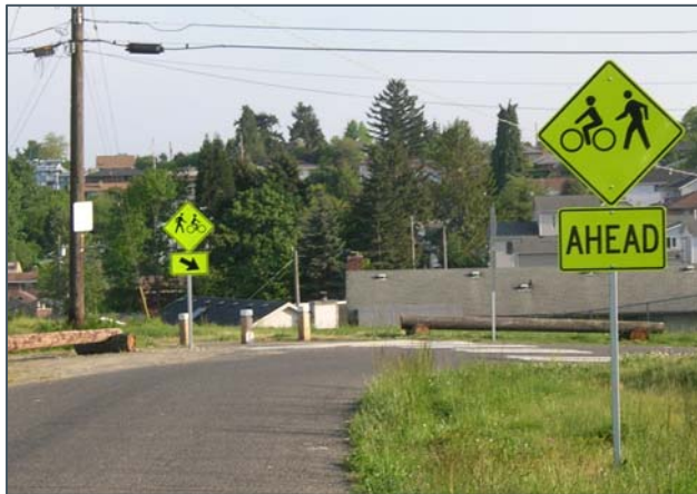
Figure H-2. Trail Warning Signs
