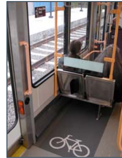
MAX light rail cars in Portland, OR have designated space for handling bicycles.
