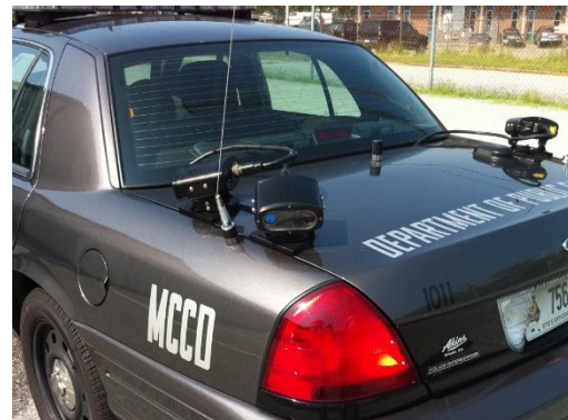
Figure 17 Mobile License Plate Readers are compact portable systems to aid in pricing enforcement
