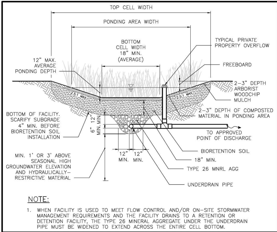
Figure 5.12. Infiltrating Bioretention Facility with Sloped Sides (with Underdrain).
