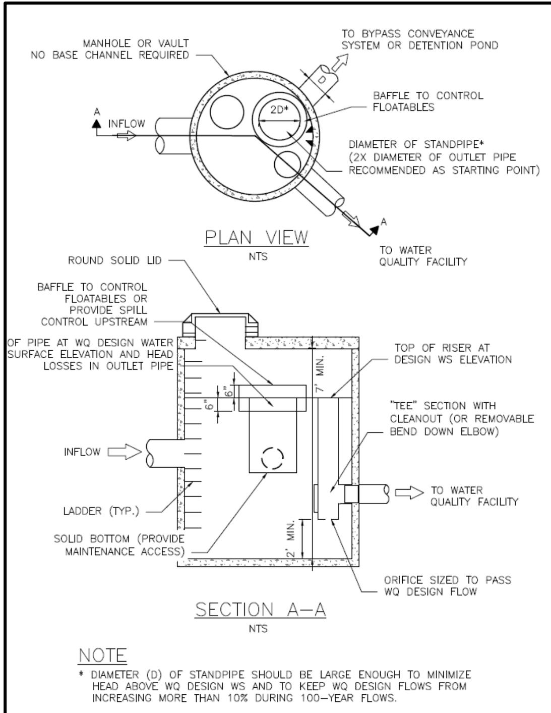
Figure E.5. Flow Splitter Example B.
