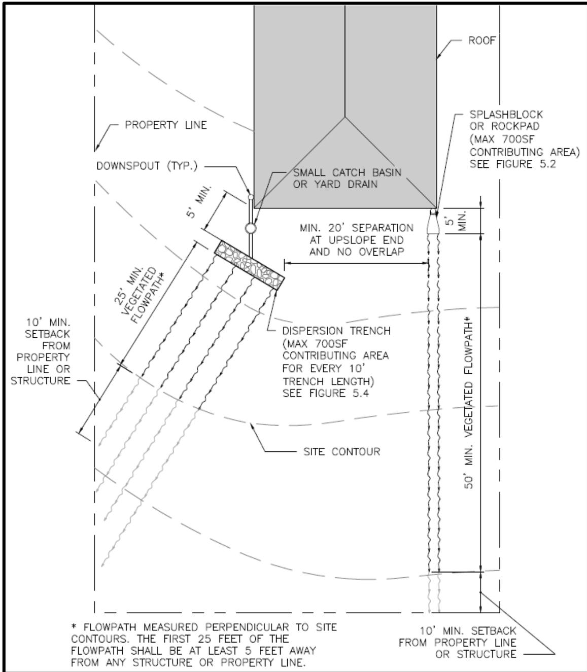
Figure 5.3. Typical Downspout Splashblock and Dispersion Trench Plan.
