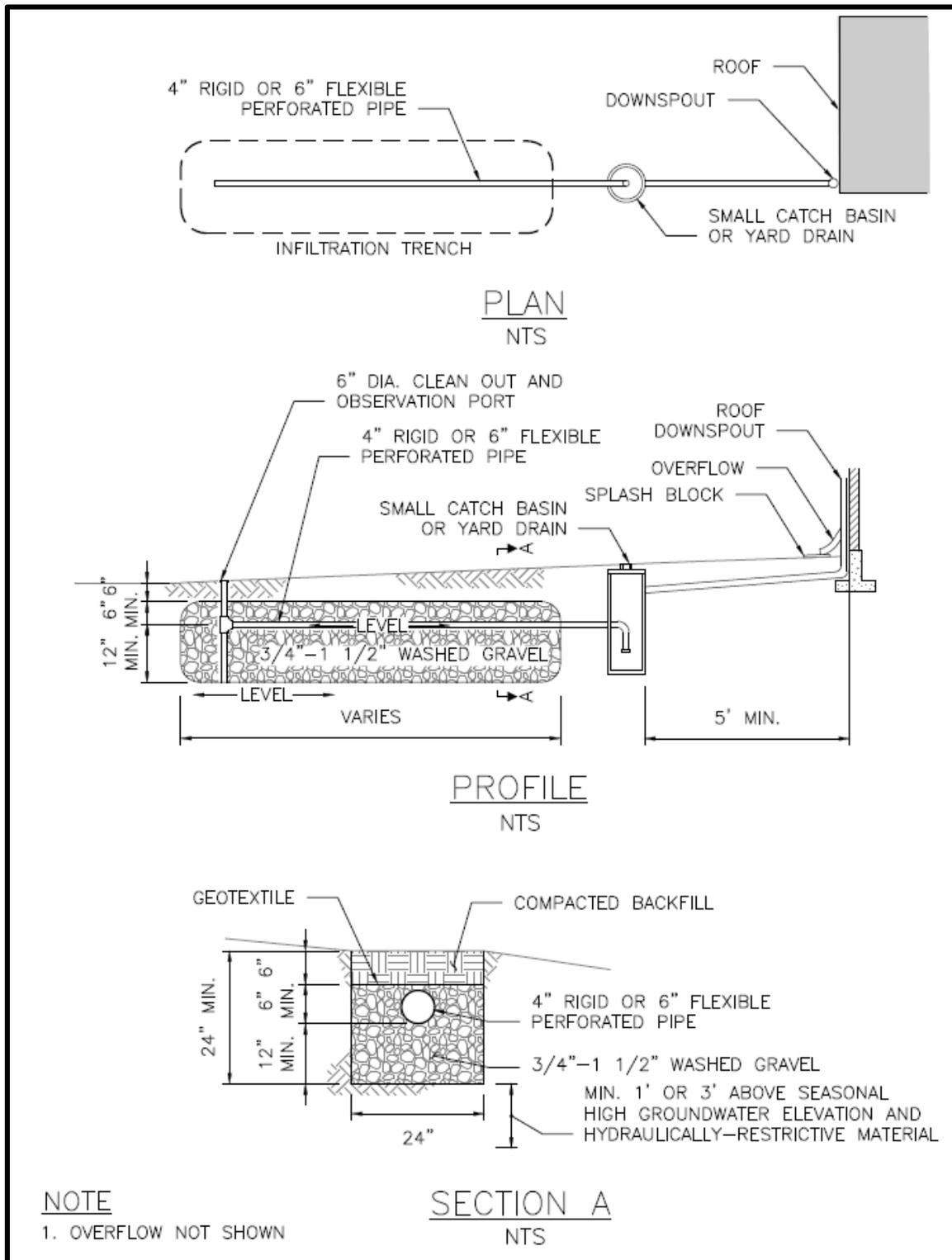
Figure 5.7. Typical Infiltration Trench Receiving Concentrated Flow.
