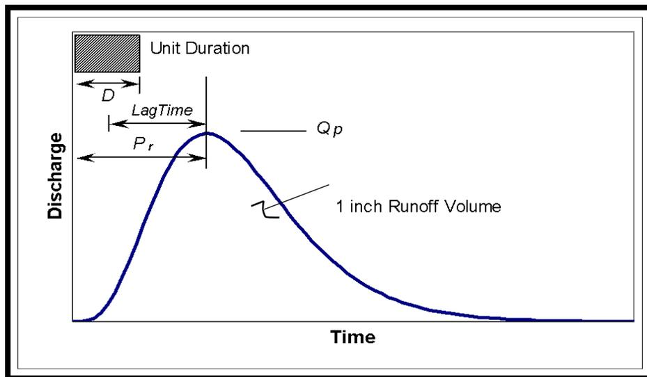
Figure F.17. Characteristics of Unit Hydrographs.
