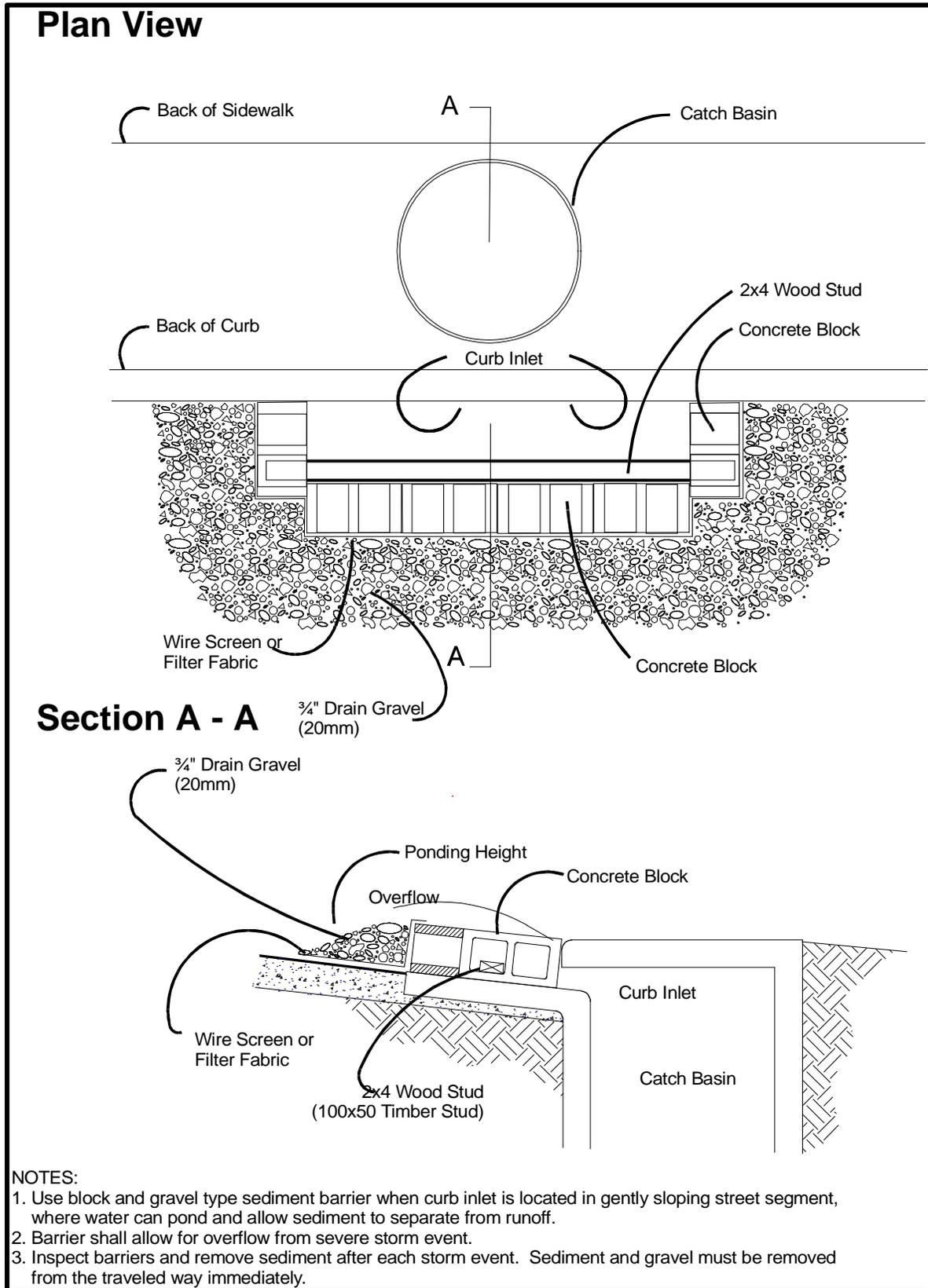
Figure 15. Block and Gravel Curb Inlet Protection.
