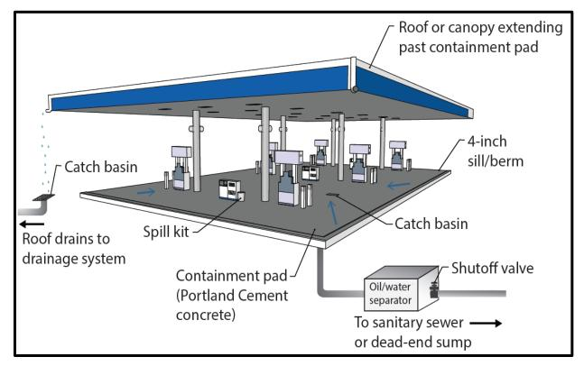
Figure 3. Fueling Island Schematic.
