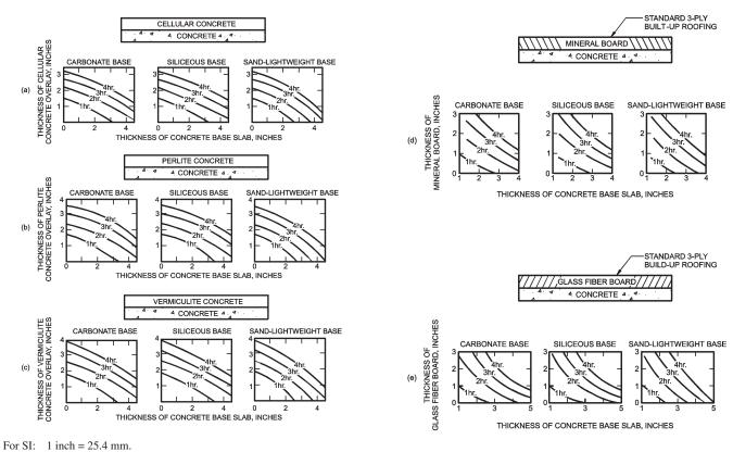
FIGURE 721.2.2.3(1) FIRE-RESISTANCE RATINGS FOR CONCRETE ROOF ASSEMBLIES For SI: 1 inch = 25.4 mm.
