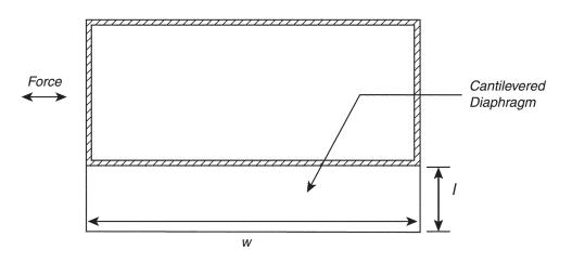
FIGURE 2305.2.5(2) DIAPHRAGM LENGTH AND WIDTH FOR PLAN VIEW OF CANTILEVERED DIAPHRAGM
