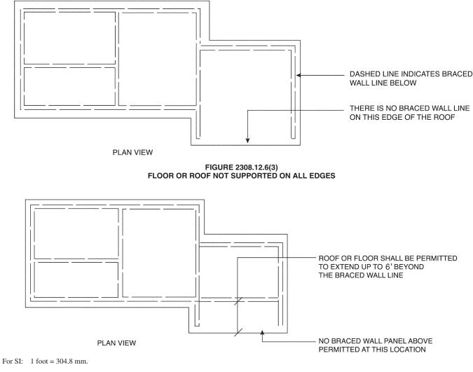
FIGURE 2308.12.6(4) ROOF OR FLOOR EXTENSION BEYOND BRACED WALL LINE
