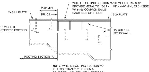
25'-0" TOTAL LENGTH WALL, PROVIDE BRACING AT CRIPPLE STUD WALL
