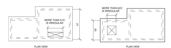
FIGURE 2308.12.6(7) BRACED WALL LINES NOT PERPENDICULAR
