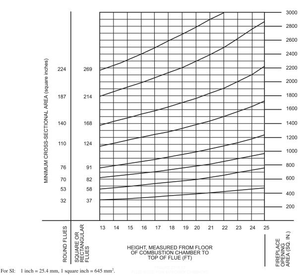
FIGURE 2113.16 FLUE SIZES FOR MASONRY CHIMNEYS
