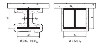
**FIGURE 721.5.2** DETERMINATION OF THE HEATED PERIMETER OF STRUCTURAL STEEL BEAMS AND GIRDERS
