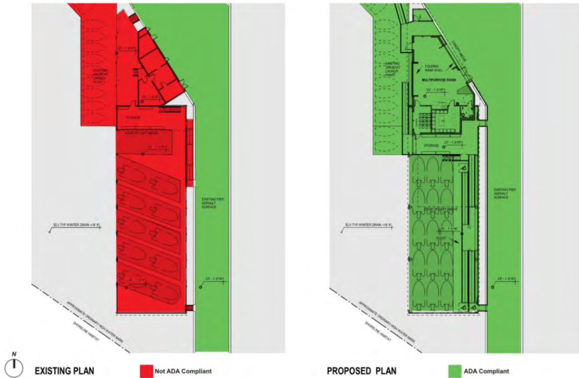
Image 33 Proposed accessibility improvements between existing and proposed building.
