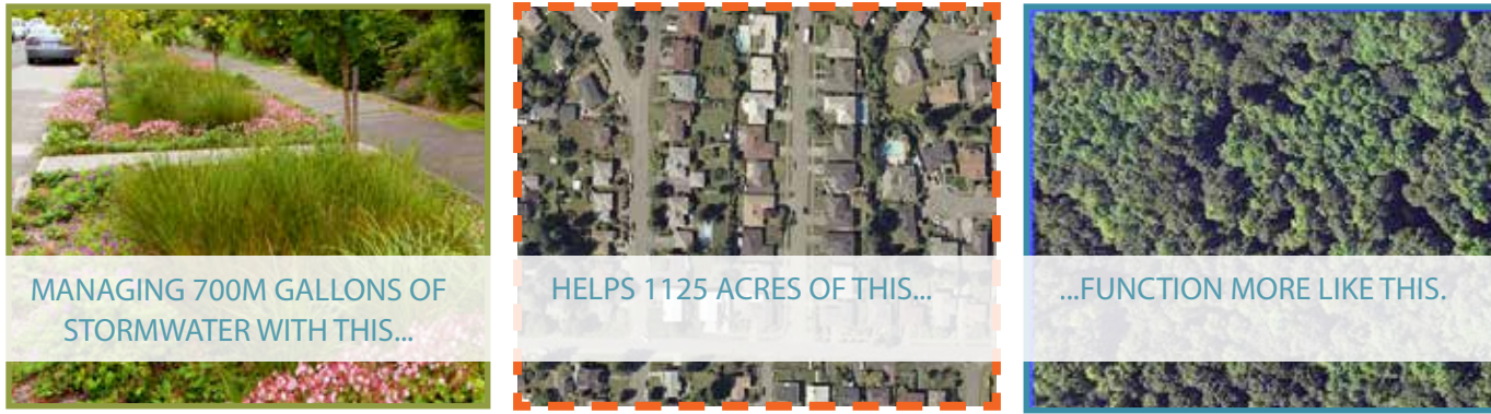
Figure 5. Managing 700M gallons of stormwater annually with GSI will help approximately 1125 acres of impervious surface in Seattle function more like a native forest.
