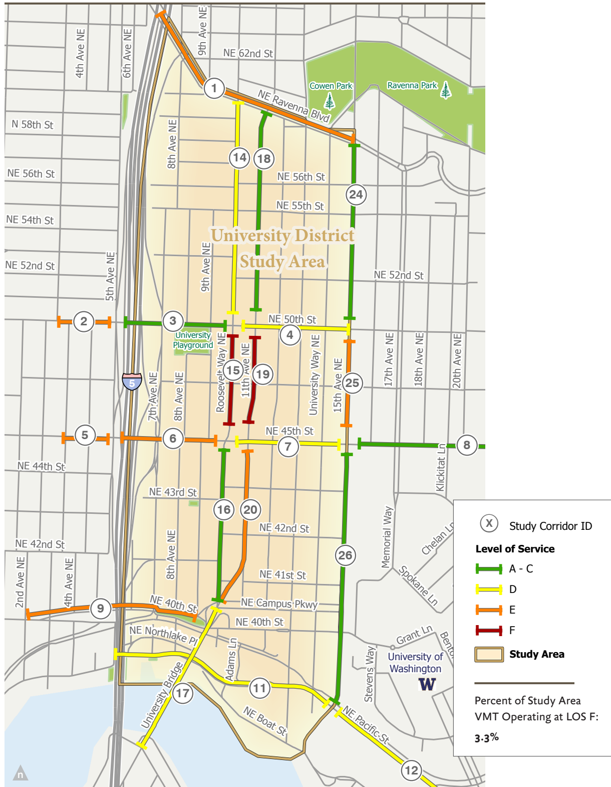
Figure 3.5–12: Auto and Freight Study Corridors—2015 Level of Service
