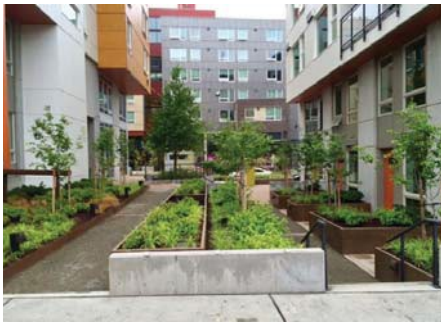
A mid-block pathway through a residential development is lined with unit entries, planters, and windows. A change in paving signifies the transition to semi-private space.
