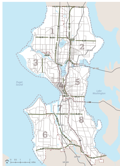
Thumbnail of Figure 3.7–16 on page 3.7–32, 2035 screenline v/c ratios. A screenline is an imaginary line across which the number of passing vehicles is counted.
