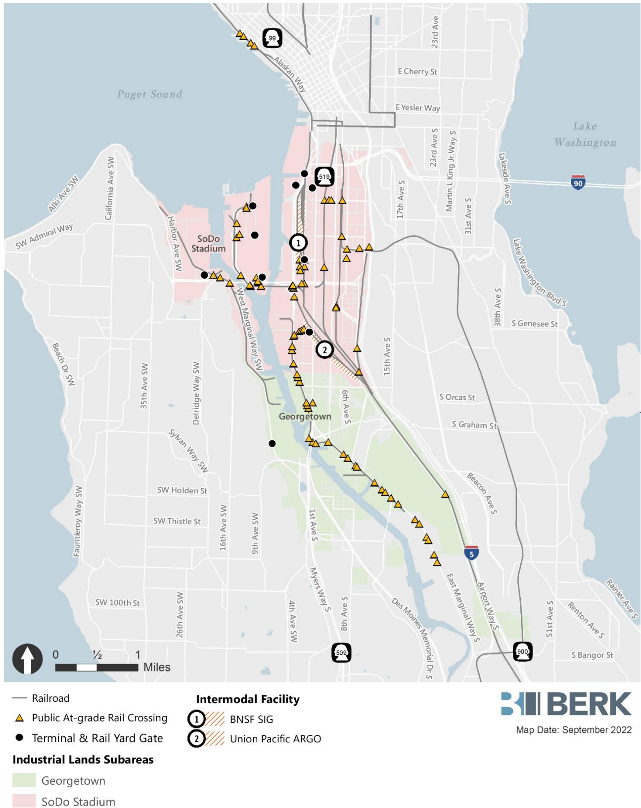
Exhibit 3.10-14 Existing Rail Freight Network—Greater Duwamish MIC, 2021
