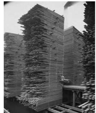
Stacks of lumber drying at the Seattle Cedar Lumber Manufacturing Company's mill in Ballard, ca. 1919
