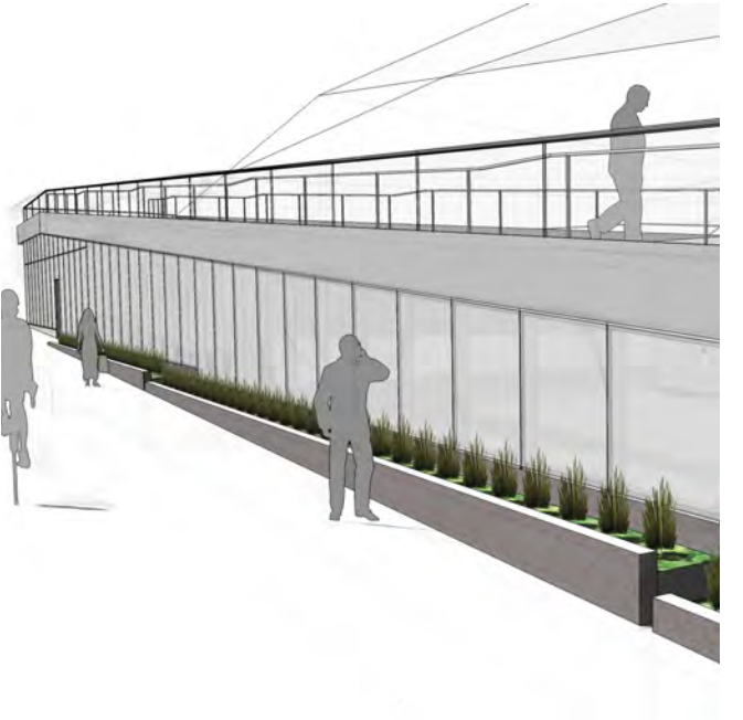
A bioretention planter treats polluted runoff generated from the alley
