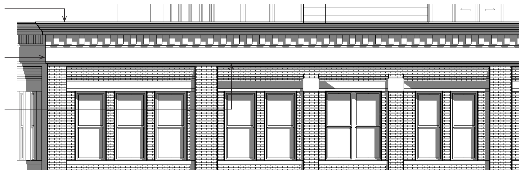
PROPOSED RECONSTRUCTED OF SOUTH BRICK PARAPET AND CORNICE
