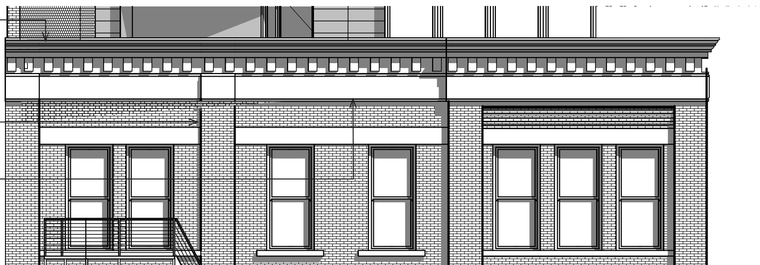
PROPOSED RECONSTRUCTED OF WEST BRICK PARAPET AND CORNICE
