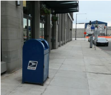
Figure xxx. This mailbox is in the pedestrian path and in the area where the visually impaired typically use their canes to navigate city streets. It should be located closer to the curb line to facilitate movement for all pedestrians.
