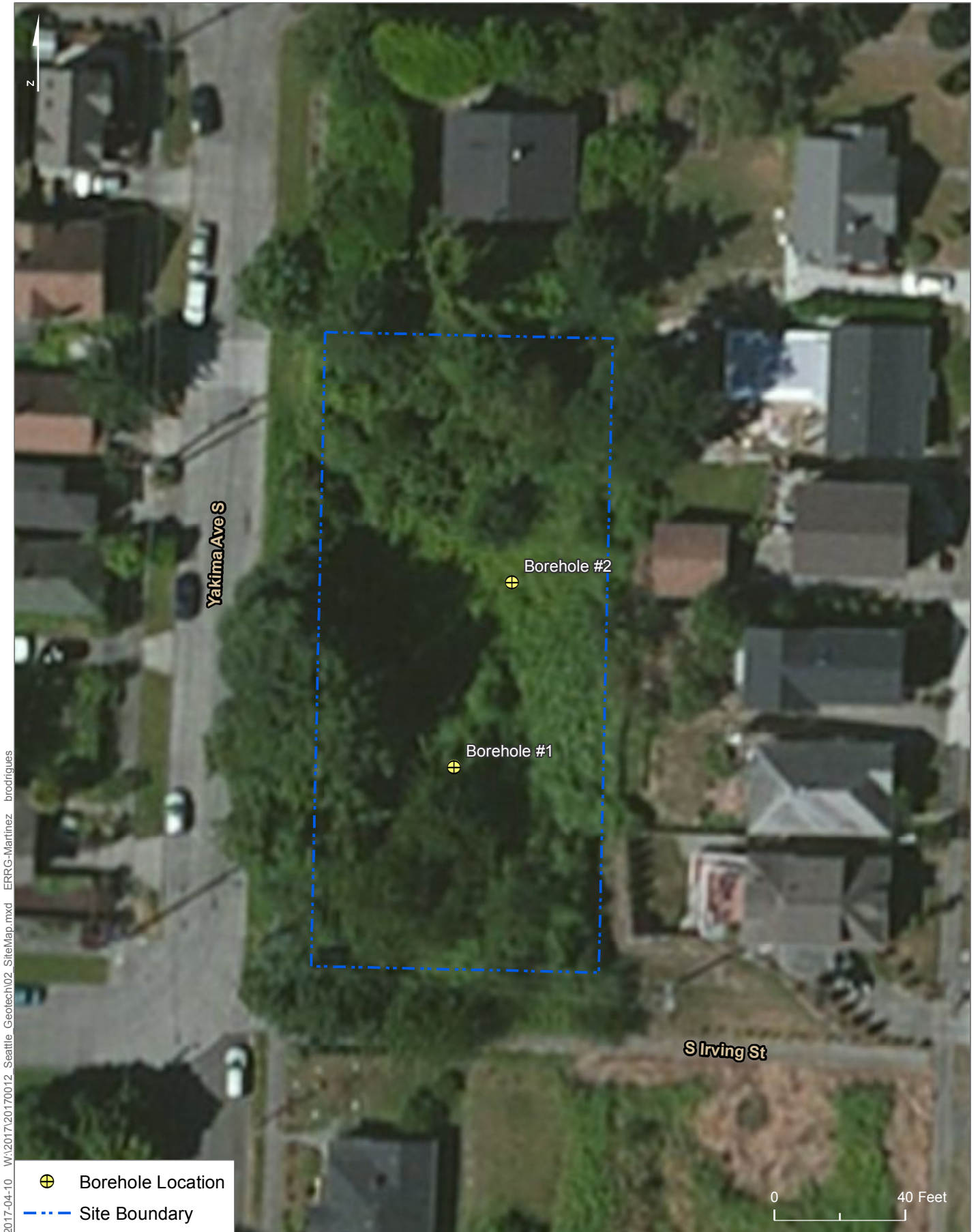
Figure 2. Site Map and Subsurface Exploration Locations City of Seattle, Washington
