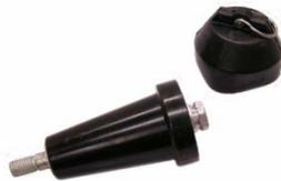
**Application:** An accessory device designed to electrically insulate, electrically shield, and mechanically seal an elbow interface. Test point cap is removable to allow access to capacitive test point. Exact same as 687270, except one loose stud is provided.
