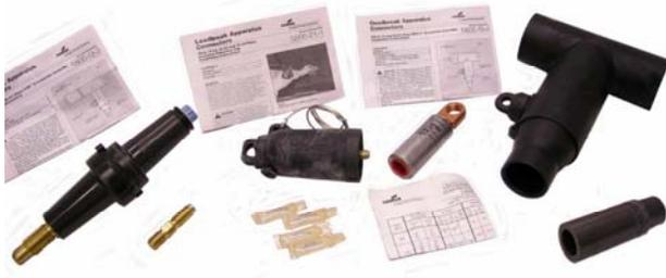
**Description:** Cooper Power Systems, 900 A, 125 kV, T-OP II, deadbreak separable connector kit, cable specific and includes T-body with test point, test point cap, cable adapter, threaded copper stud, copper compression connector, and insulated cap for 200 A bushing.
