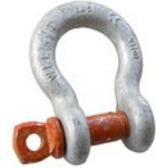
Anchor shackles with screw pins can be used in side-loading situations; however users should be aware that this reduces effective working load limits.
