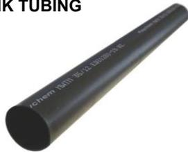
**Application:** Medium wall heat shrink tubing is applied over broken-out, taped-shielded cable to provide mechanical and environmental protection. Cables of this type are exclusive to the Network system. Medium wall heat shrink tubing may also act as primary insulation for systems rated 600 volts and below. Product is considered non-flame retardant. Use only an approved propane torch, Stock Number 765897, to install heat shrink products.
