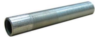
**Description:** UL 6 defines a nipple to be a straight section of conduit 24 inches in length or less, with male pipe threads at each end. SCL purchases nipple stock, also known as running thread, in 3-ft lengths.
