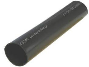
**Application:** Splice covers, also known as shrink tubes or shrinks, are used to seal, insulate, and protect cable joints and terminations. They are appropriate for submersible and direct burial installations. Splice covers may also act as primary insulation for systems rated 600 volts and below. Product is considered non-flame retardant. Use only an approved propane torch, Stock Number 765897, to install heat shrink products.
