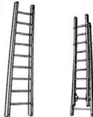
**Application:** Wood ladders are used by operations personnel to access underground vaults and above ground structures. Highest standing levels are below. Maximum intended load is 300 pounds.
