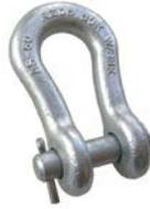
Anchor shackles with round pins can be used in tie down, towing, suspension or lifting applications where the load is strictly applied in-line. Round pin shackles should never be used in rigging applications to gather multiple sling legs, or where side loading conditions may occur.
