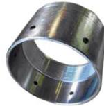
**Description:** Zinc-coated steel. Set-screw type, steel couplings are used to join threaded sections of 5-in steel conduit to straight-cut, unthreaded sections. These are used where it is not practical or possible to use a standard, 5-in threaded coupling, Stock No. 731102. This coupling also satisfies federal "Buy American" policies.
