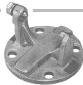
**Application:** This adapter is used to convert a standard 115 kV polymer station post insulator (Stock No. 012383) to a vertical line post insulator with a trunnion end fitting. Use bracket Stock No. 693017 to mount insulator to pole top.
