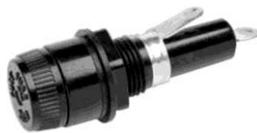
Panel-mount fuse holders are intended for mounting in panel holes 0.505 +/- .005 inches in diameter.
