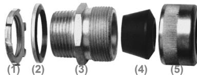
**Description:** complete connector with locknut (1), sealing gasket (2), body (3), Neoprene bushing (4), and gland nut (5)
