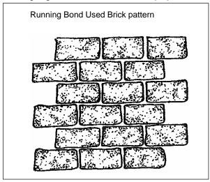
The Contractor must use the Running Bond Used Brick pattern for crosswalks or at other locations when shown on the Drawings.
