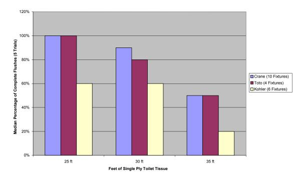
Median Flushing Performance of (20) Fixtures with 1.5 gpf Gem II Flush Valve 75-85 psi Static / 30-40 psi Flowing
