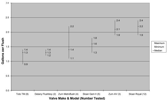
Flush Volumes for Tested Valves 70 psi Static
