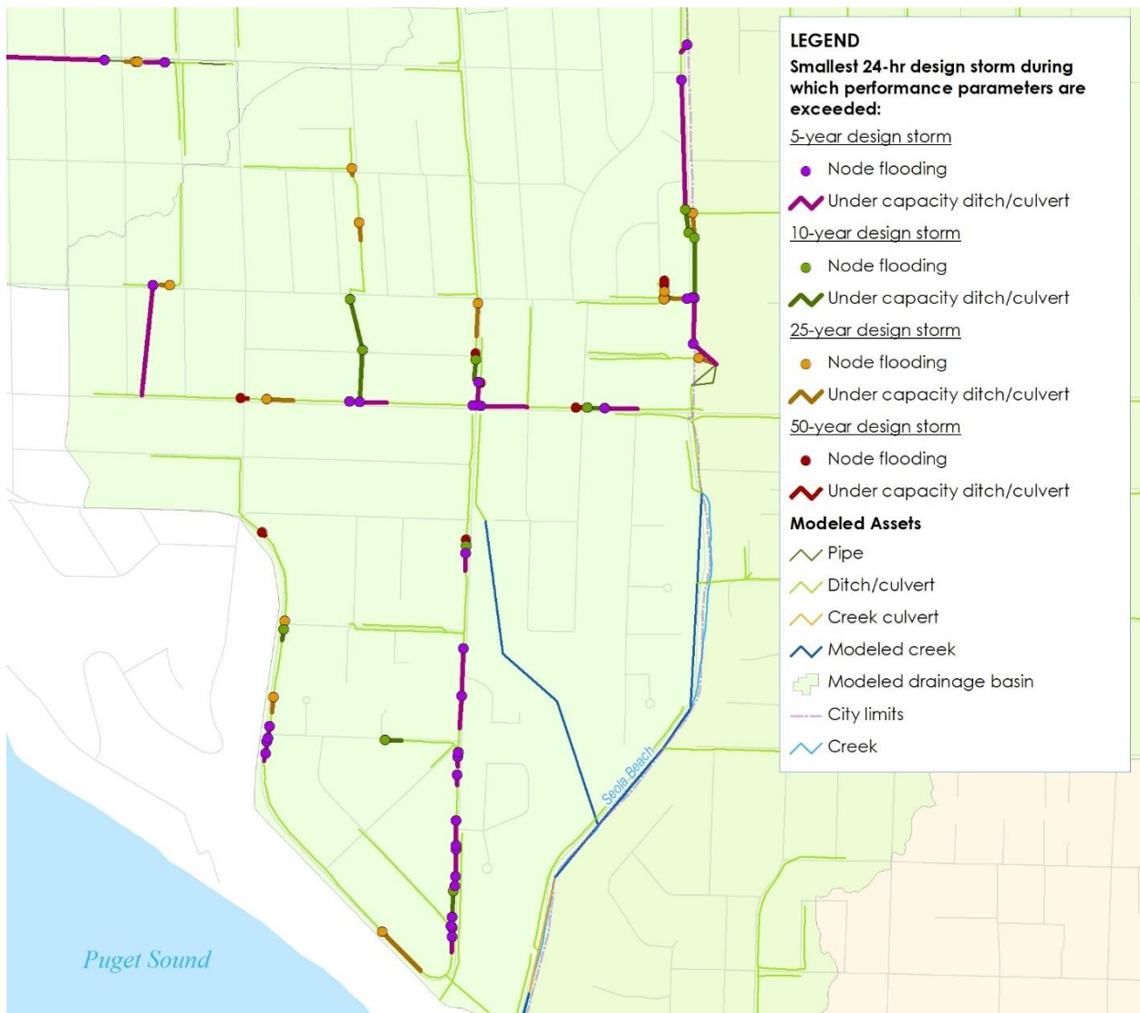
Figure 9. Example of the ditch and culvert drainage system simulated for capacity evaluation
