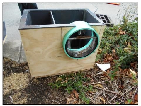
Pressure transducers (Campbell Scientific Inc. CS451-L) were installed in a stilling chamber to monitor water depth upstream of the weir in the outlet chamber.
