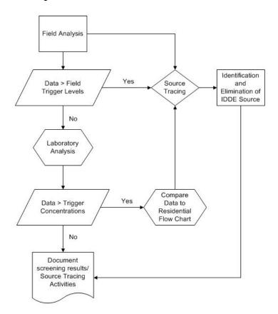
Figure III.8-1. IDDE Field Screening Flow Chart
