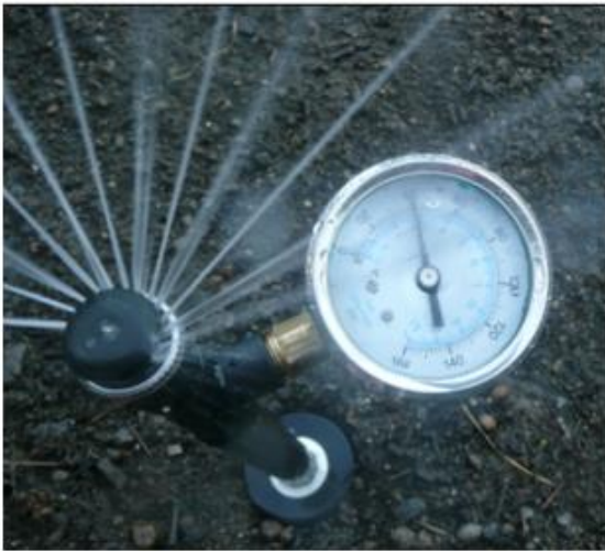
Photo 1. 40 psi after adjustments to Zone 9 (most west zone in south lawn panel) on 10/11/12
