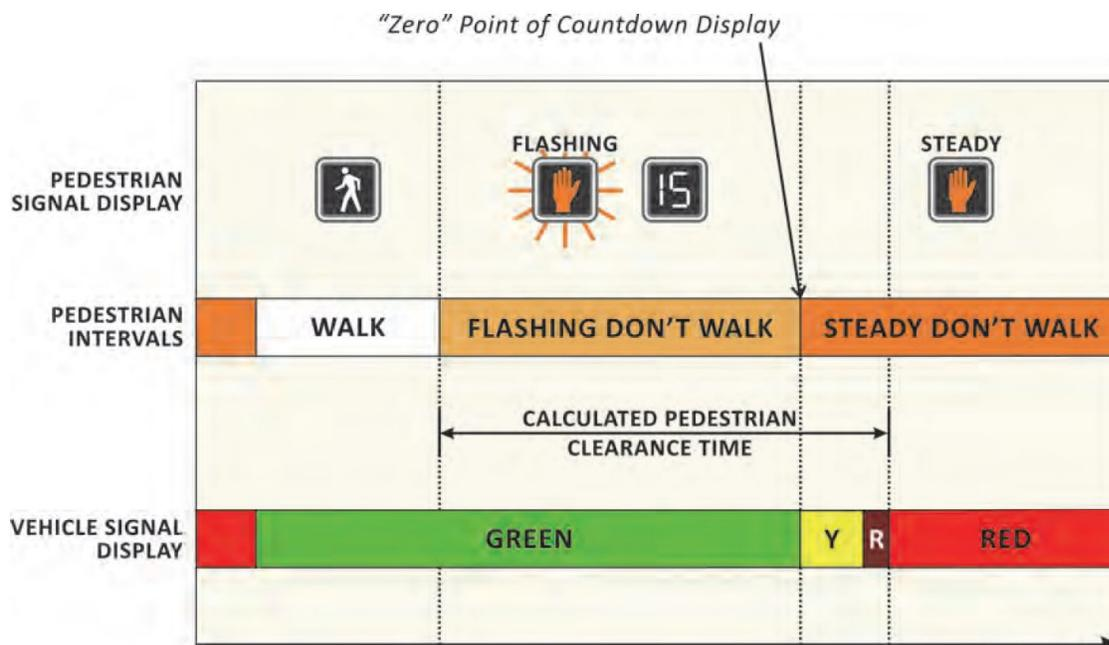
Figure 1 Pedestrian Interval (NCHRP Report 812-Signal Timing Manual 2nd Edition)
