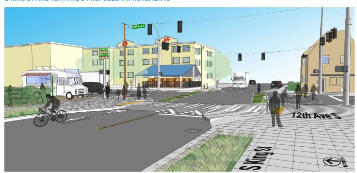
Adding a raised crosswalk, curb ramps, bike ramps, and crossing signals at S King St and 12th Ave S will help increase the visibility of people walking and biking and make it a safer intersection.
