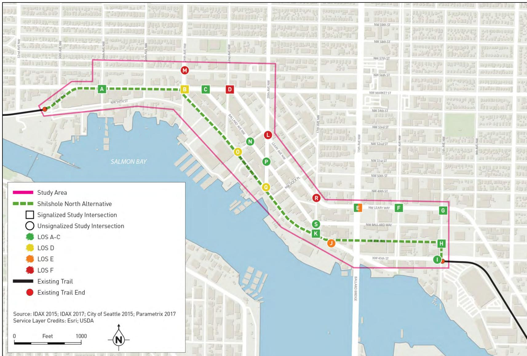
Figure 7-14. Shilshole North Alternative PM Peak Hour Study Intersection Level of Service
