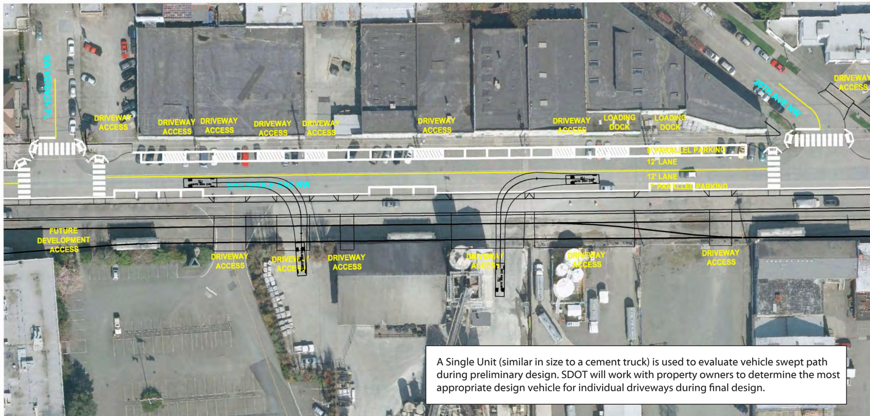
A Single Unit (similar in size to a cement truck) is used to evaluate vehicle swept path during preliminary design. SDOT will work with property owners to determine the most appropriate design vehicle for individual driveways during final design.
