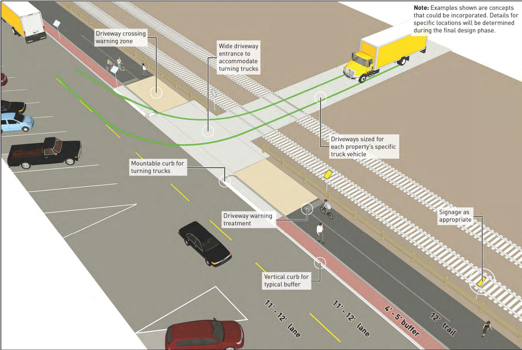
Figure 1-8. Intersection Design Options: Curb Radii Modification
