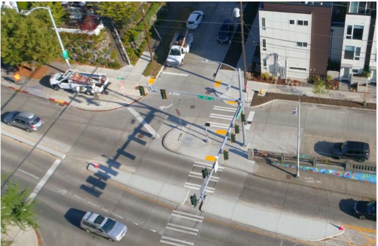
Program 18 – Aerial view of N 46th St and Aurora Ave N, showing an expanded bus stop, new signalized crosswalk, curb ramps and sidewalk upgrades, repaving, pedestrian lights, westbound protected left turn, and much more. This intersection was one of many improved as part of the Route 44 Transit Plus Multimodal Corridor project.
